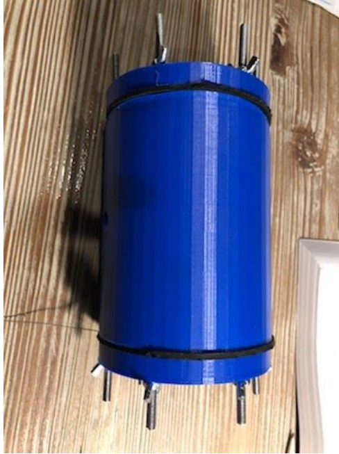
Fig 6. Flat Anode MFC Assembled
