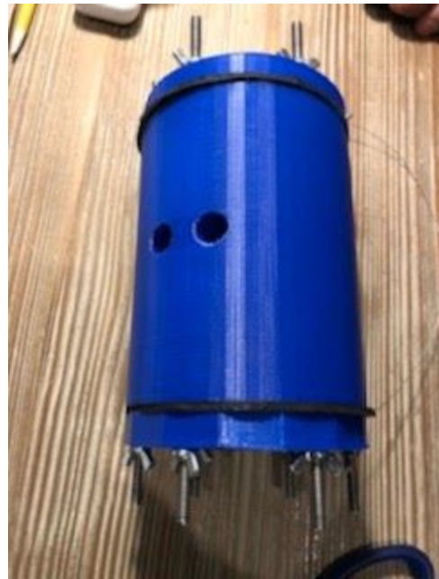
Fig 7. Curved Anode MFC Assembled
